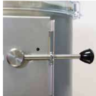
Water inlet system with non-return air break.
