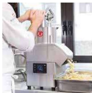
Vegetable slicer function: lateral product ejection.
