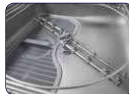
Secondary wash tank filters
